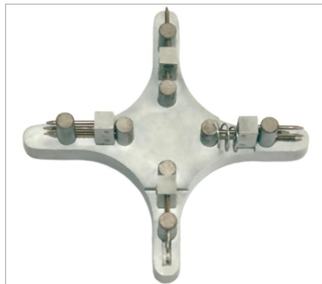
Figure 1 - Prototype of bracket-positioning gauge.
