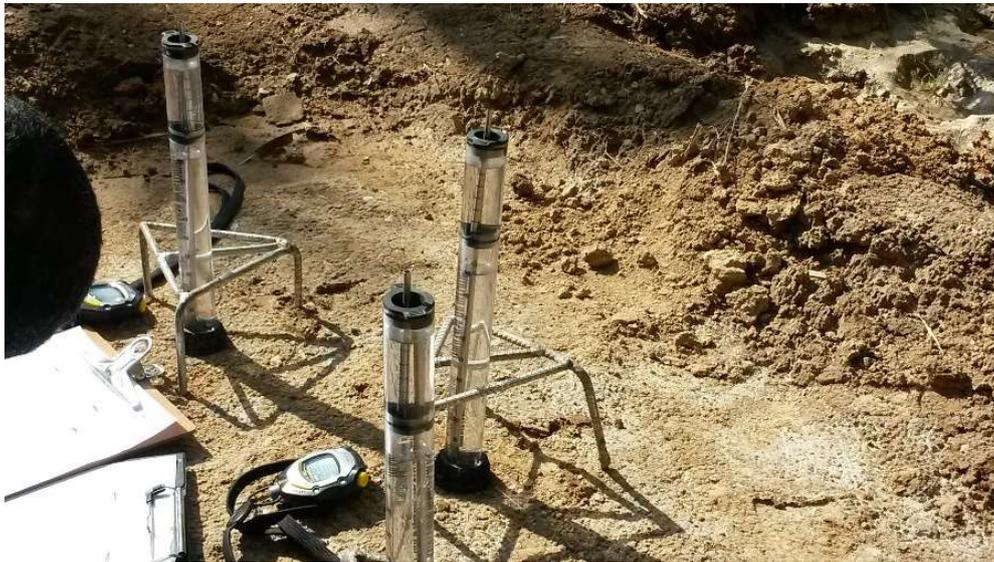
FIGURE 1. Mini disk infiltrometer used for field infiltration measurements.
