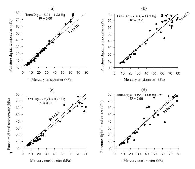
FIGURE 3. Regression and correlation analysis between the soil water matric potential (module) by mercury tensiometer and puncture digital tensiometer in plots P1 (a) P2 (b), P3 (c) and P4 (d).
