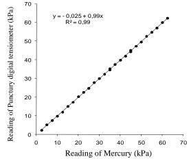
FIGURE 1. Calibration of digital tensiometer reading system.
