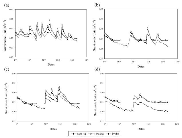
FIGURE 4. Mean values from gravimetric soil moisture measured by mercury tensiometer (Tens Hg), puncture digital tensiometer (Tens Dig) and neutron probe (Sonda) in plots P1 (a) P2 (b), P3 (c) and P4 (d).
