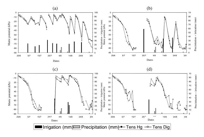
FIGURE 2. Soil water matric potential measured by the mercury tensiometer (Tens Hg) and puncture digital tensiometer (TensDig) in plots P1 (a) P2 (b), P3 (c) and P4 (d).
