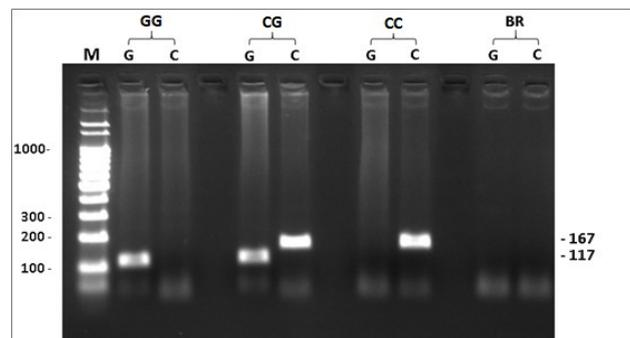
**Figure 1** – Electrophoretic pattern of allele specific PCR of rs527616 (C>G), located in the lncRNA *AQP4-AS1*. M: Molecular weight marker, GG: Homozygous sample, CG: heterozygous sample, CC: homozygous sample, BR: white control. Expected fragment size: C-167 bp and G-117 bp.
