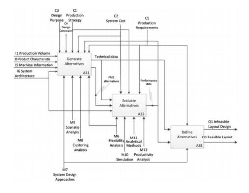
Figure 9. IDEF modeling: context diagram layout design and performance appraisal. Source: Pinarbaşi et al. (2013).
