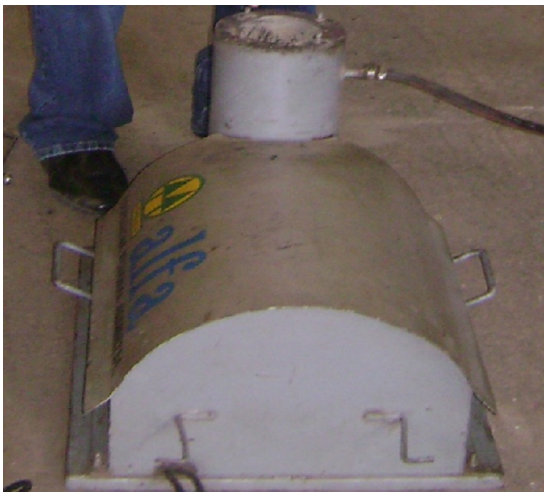
Figure 4. Experimental scale model used for the simulation of explosions. Source: Developed by the authors.
