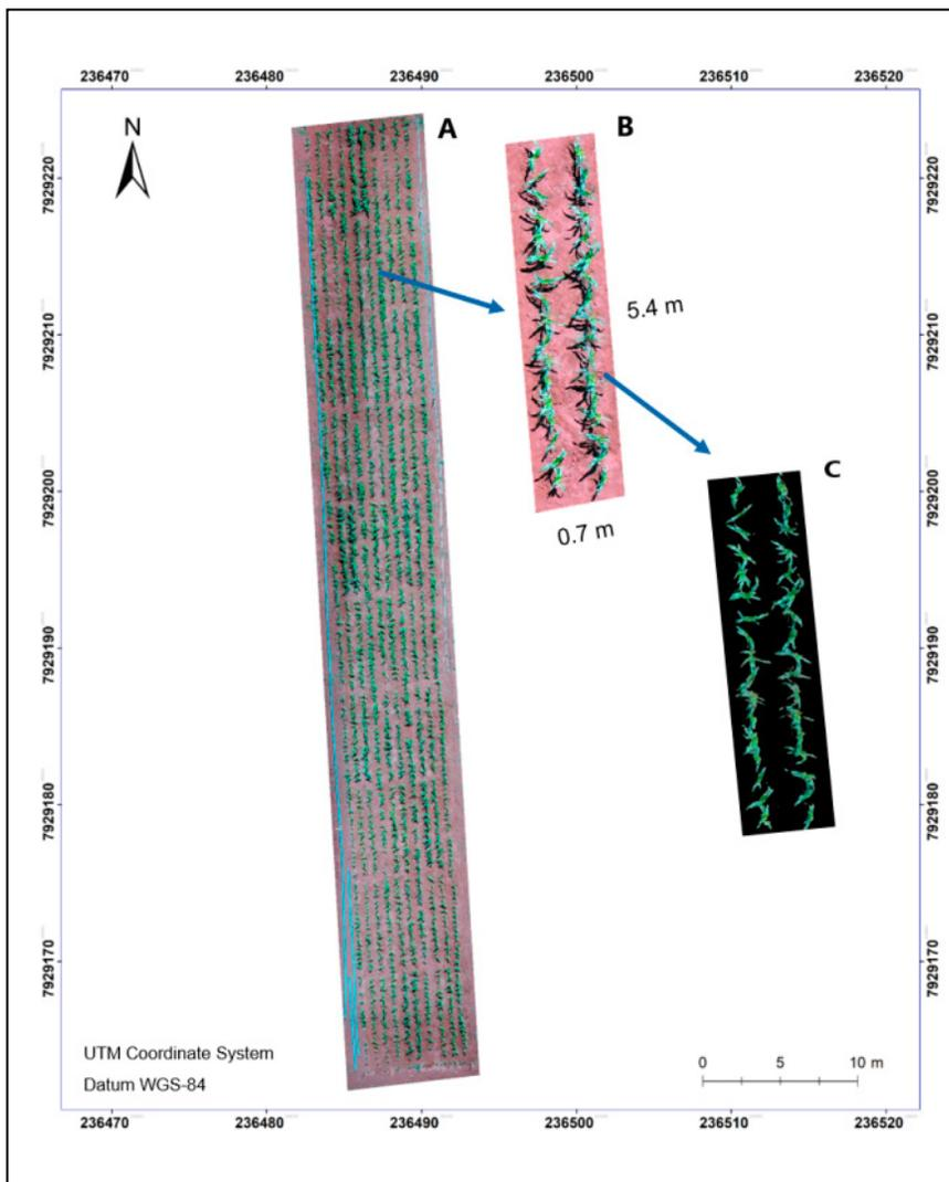
**Figure 1.** Experimental setup. **A.** Aerial image mosaic of the experiment with plots of sweet corn hybrids, captured with an unmanned aerial vehicle platform; **B.** the experimental setup with single plot details; and **C.** plot image segmentation by the k-means clustering algorithm. Monte Carmelo, UFU, 2021.
