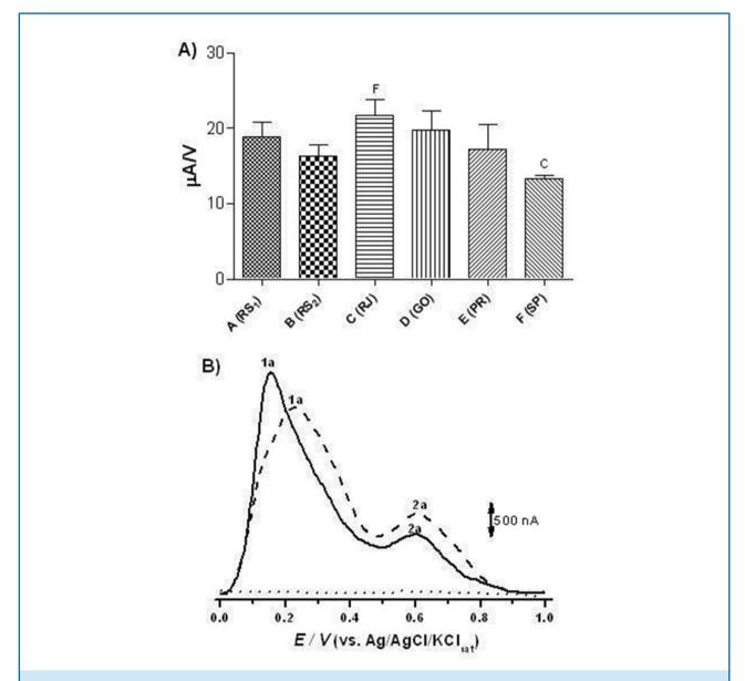
Figure 2 - Electrochemical Index (EI) chart representing the sum of the  $I_{pa}/E_{pa}$  (A) rates and differential pulse voltammograms (B) obtained using carbon paste electrode for analysis of C (RJ) (—) and F (--) (SP), which presented the highest and the lowest potential of antioxidant activity, respectively. The white (...) was achieved in 0.01 M pH 7 sodium phosphate buffer.
