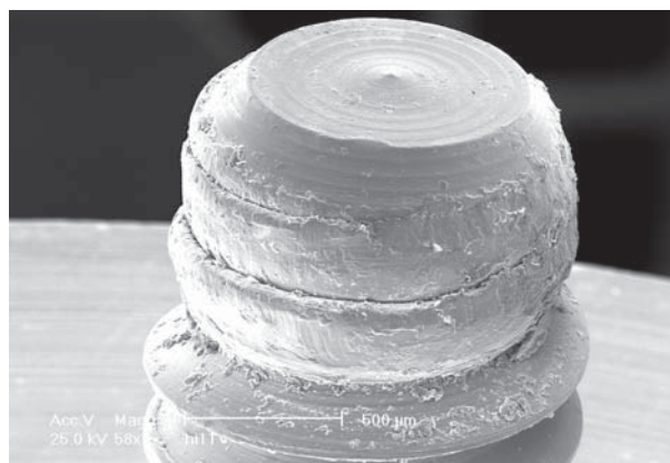
Figure 5- Scanning electron microscopy (SEM) micrograph demonstrating damages in the screw threads without fracture
