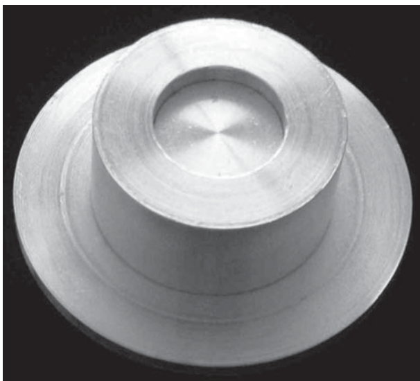
Figure 1- Metallic matrix with 15-mm diameter and 2-mm thickness
