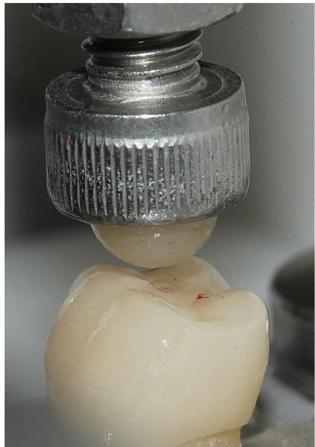
**Figure 1-** Position of indenter during fatigue test
