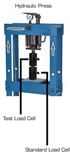
Figure 6. Arrangement for Pre-Test Load Cell Verification.
