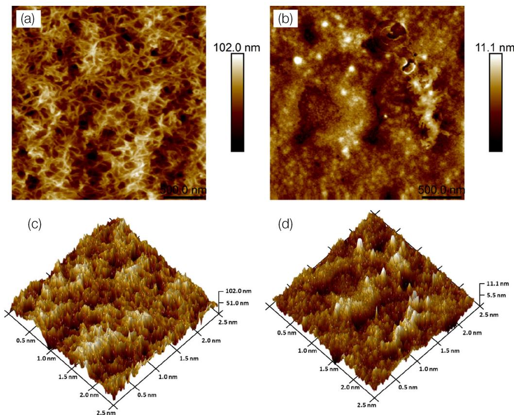
**Figure 2.** Topographic AFM maps (2  $\mu\text{m}$  scan size) of the PDN-a (a) and PDN-s (b) samples and their respective three-dimensional maps (c, d). The scale bars represent the heights (maximum values) of the structures observed in the images.
