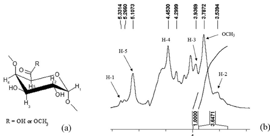
**Figure 1.** Chemical structure of the monomer unit of pectin (a) and expansion of a region of the  $^1H$  NMR spectrum (300 MHz,  $D_2O$ ) of PDN-a sample showing the peak integrals used for DM estimation (b).
