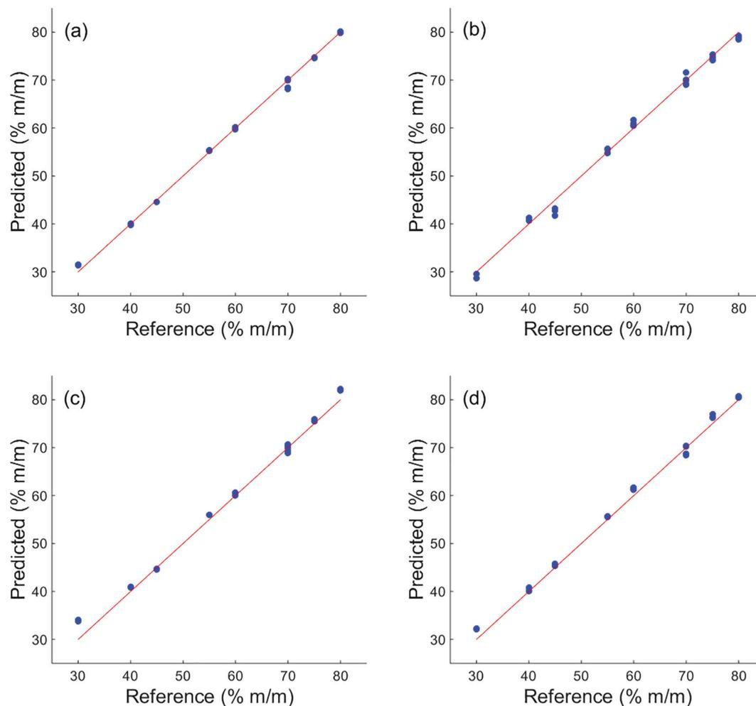
**Figure 2.** Predicted *versus* reference plots for the prediction set using type 2 PLS models in the (a) MIR and (b) NIR ranges and univariate models in the (c) MIR and (d) NIR ranges. The line shown is the quadrant bisectrix.
