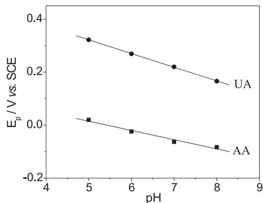
**Figure 6.** Dependence on pH of the peak potentials ( $E_p$ ) for  $100 \text{ } \mu\text{mol L}^{-1}$  AA and  $100 \text{ } \mu\text{mol L}^{-1}$  UA in the presence of  $1.0 \text{ mmol L}^{-1}$  CPC.
