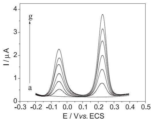
**Figure 5.** Differential pulse voltammograms (DPV) for the mixture of AA and UA in  $0.1 \text{ mol L}^{-1}$  phosphate buffer (pH 7.0) and in micelle media ( $1.0 \text{ mmol L}^{-1}$  CPC). Concentrations of both AA and UA are simultaneously changed: (a) [AA] and [UA] 0; (b) [AA] 20 and [UA] 10; (c) [AA] 40 and [UA] 20; (d) [AA] 60 and [UA] 30; (e) [AA] 80 and [UA] 40; (f) [AA] 100 and [UA] 50; (g) [AA] 120 and [UA]  $60 \text{ } \mu\text{mol L}^{-1}$ .
