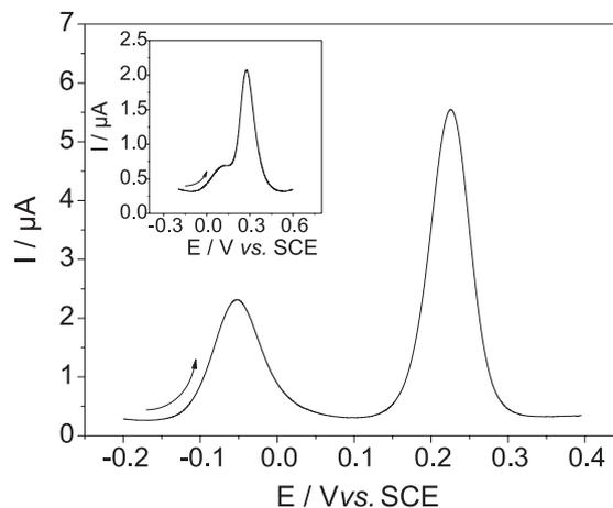
**Figure 3.** Differential pulse voltammograms (DPV) for the mixture of a solution of  $100 \mu\text{mol L}^{-1}$  AA and  $100 \mu\text{mol L}^{-1}$  UA in  $0.1 \text{ mol L}^{-1}$  phosphate buffer (pH 7.0) and in micelle media ( $1.0 \text{ mmol L}^{-1}$  CPC). Inset graphic shows the response for oxidation of AA and UA in the absence of CPC, both coexisting in solution. Potential amplitude was  $50 \text{ mV}$ . Step potential of  $5 \text{ mV}$ .
