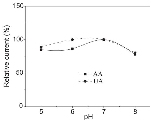
**Figure 7.** Dependence on pH of the peak currents ( $I_p$ ) for  $100 \mu\text{mol L}^{-1}$  AA and  $100 \mu\text{mol L}^{-1}$  UA in the presence of  $1.0 \text{ mmol L}^{-1}$  CPC. Currents data was showed as a relative response.
