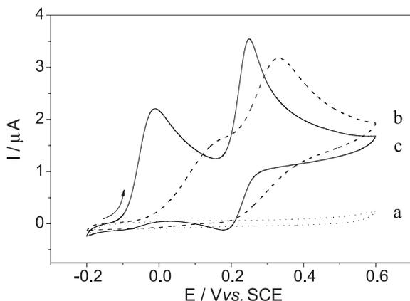
**Figure 2.** Cyclic voltammograms of mixtures of  $100 \mu\text{mol L}^{-1}$  AA and  $100 \mu\text{mol L}^{-1}$  UA recorded at a glassy carbon electrode in a  $0.1 \text{ mol L}^{-1}$  phosphate buffer solution (pH 7.0). Curve a (dotted line): in  $1.0 \text{ mmol L}^{-1}$  cetylpyridinium chloride (CPC) and in the absence of both AA and UA; curve b (dashed line): AA + UA in the absence of CPC; curve c (solid line): AA + UA in the presence of CPC.  $v = 50 \text{ mV s}^{-1}$ .
