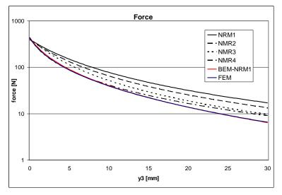
Fig. 20. Magnetic force developed by the actuator changing parameters x1 and x3.
