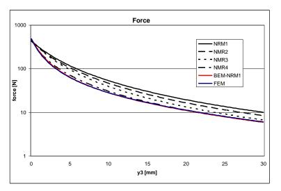
Fig. 18. Magnetic force developed by the actuator.
