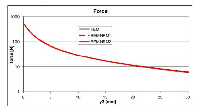
Fig. 9. Magnetic force developed by the actuator.
