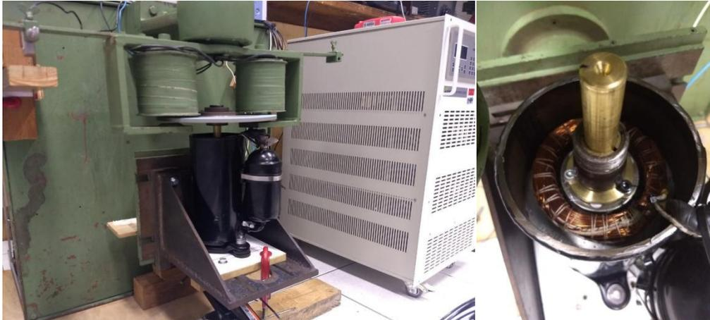
Fig. 8. Motor 5 and test bench adapted for vertical testing (left) and shaft extension (right).
