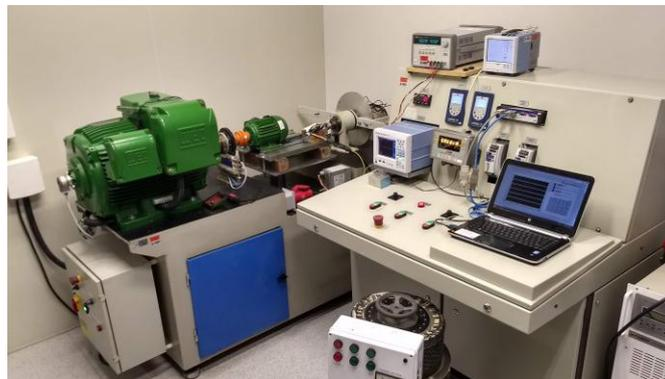
Fig. 6. Test bench for electric motors.
