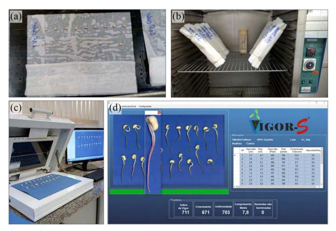
Figure 1. Steps for computer analysis: installation of the seed germination test (a); substrate positioned at a nearvertical angle (75 to 85° from the horizontal axis) (b); image acquisition by an inverted scanner (c) and analysis window of cowpea seedlings scanned and processed by the software Vigor-S (d).
