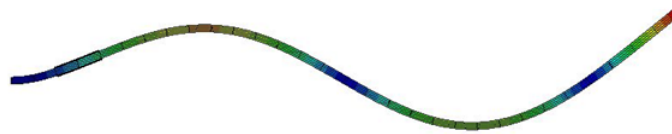
Figure 11 Mode shape of beam (a) using 2D-FE (ABAQUS)
