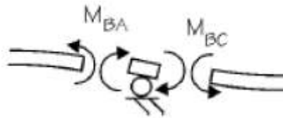
Figure 2: Free-body diagram for moment at node B (Lopes et al., 2011).
