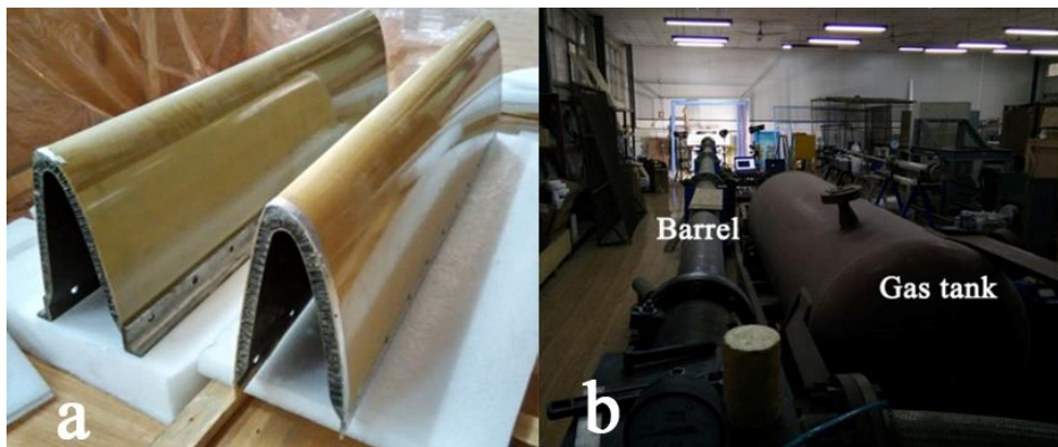
Figure 12: Birdstrike experiment, (a) wing leading edge, (b) air-gun.
