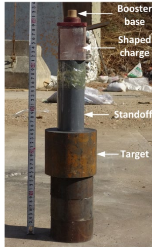
Figure 4 Experimental setup of DOP tests
