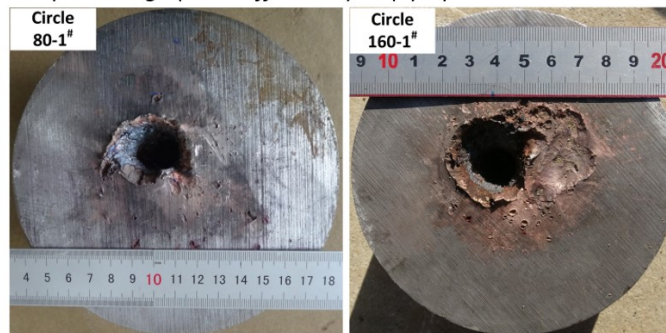
(c) circular cross-section shaped charge
