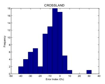
Figure 1: Histogram of fatigue index error for Crossland criterion.
