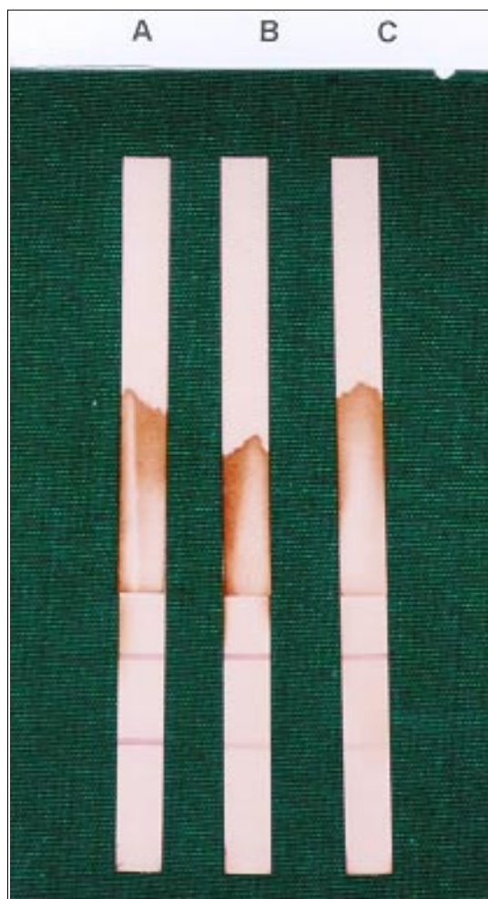
Three dip stick results which the intensity of the colour varied according to the parasitemia level, the color of the line was distinct when the level of parasitemia was high (A) whereas in the case of a low level of parasitemia, a pale positive line appeared (C, B).
