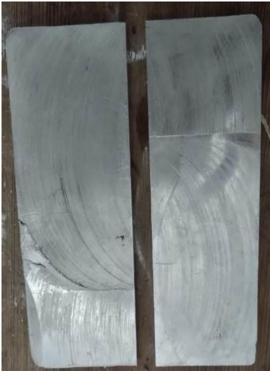
Figure 1. The fabricated stir cast AA6092/ B 4 C composite plate.
