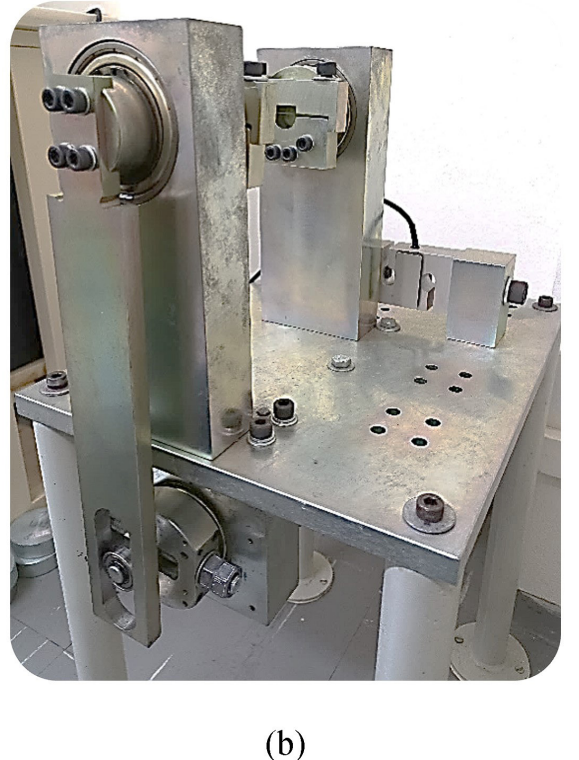
Figure 2. (a) Illustration of mechanism known as Scotch Yoke. (b) Torsional fatigue machine used in this study.
