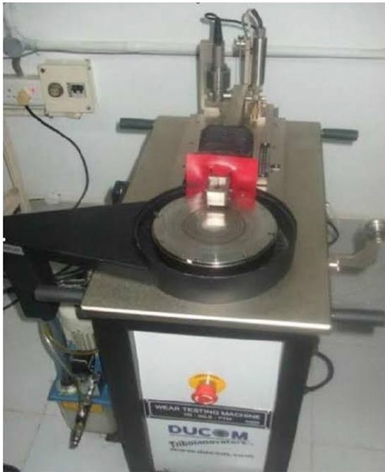
Figure 4. Wear testing machine.
