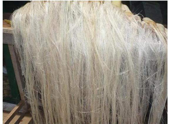
Figure 3. Pineapple fibers, PALF, extracted from the leaves of Ananas cosmos .
