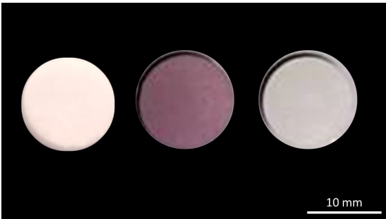
Figure 5. ICE-Zirkon (left), ZTA-Cr 2 O 3 (middle), and ZTA-MgO (right) specimens.
