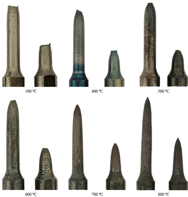
Figure 6. Specimens after the high temperature tensile tests of the Premium rail steel.
