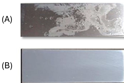
Figure 4. Photographs of the surfaces of the AISI 1020 carbon steel samples after adsorption of the inhibitors: (a) commercial and (b) natural based on limonene.
