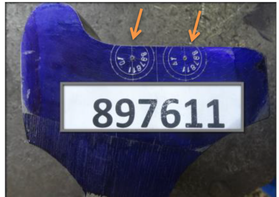
Figure 3. Location of the specimens for tests
