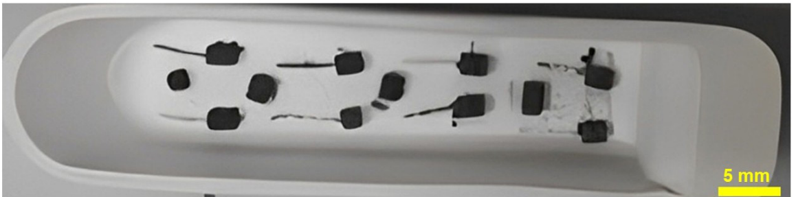
Figure 2. Green compacts of niobium powder – electrodes.
