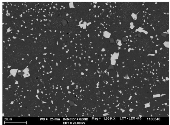
**Figure 9.** SEM of M3:2; 1180 °C/540 °C.
