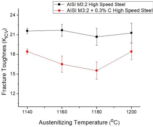
**Figure 4.** Fracture toughness (K<sub>ICV</sub>) test results of vacuum sintered AISI M3:2 high speed steel.
