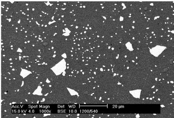
Figure 11. SEM of M3:2; 1200 °C/540 °C.
