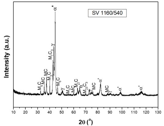
**Figure 8.** XRD of M3:2; 1160 °C/540 °C.
