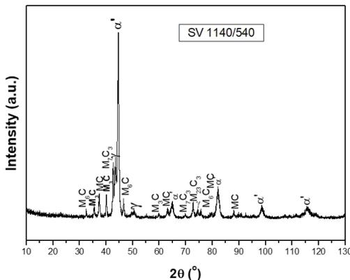
**Figure 6.** XRD of M3:2; 1140°C/540°C.
