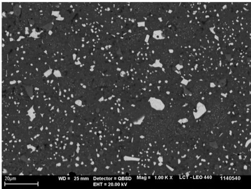
**Figure 5.** SEM of M3:2; 1140°C/540°C.
