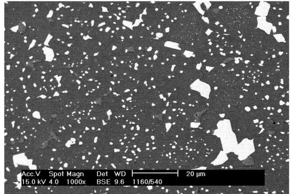
**Figure 7.** SEM of M3:2; 1160 °C/540 °C.
