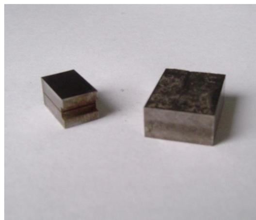
**Figure 2.** Chevron notch specimen machined from fractured TRS specimen.
