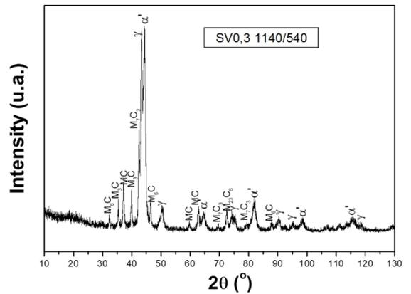
Figure 14. XRD of M3:2; 1140 °C/540 °C.
