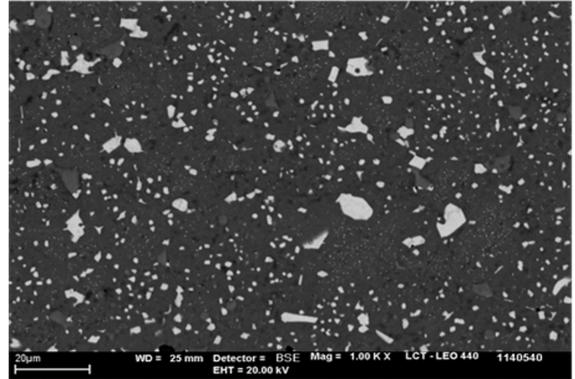
Figure 13. SEM of M3:2; 1140 °C/540 °C.
