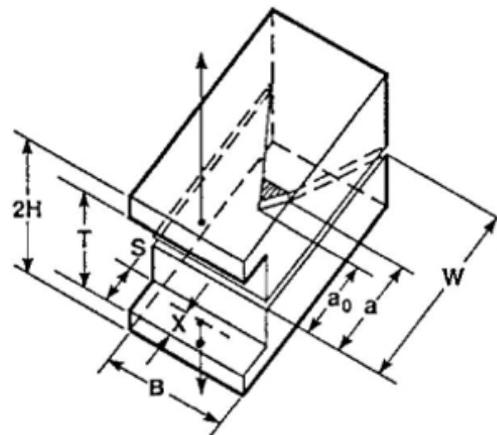
**Figure 1.** Geometry of fracture toughness test specimens, as per Chevron methodology.
