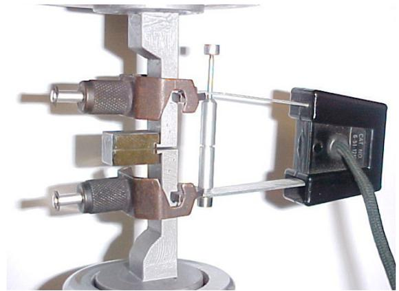
Figure 3. Apparatus used in the KICV test.
