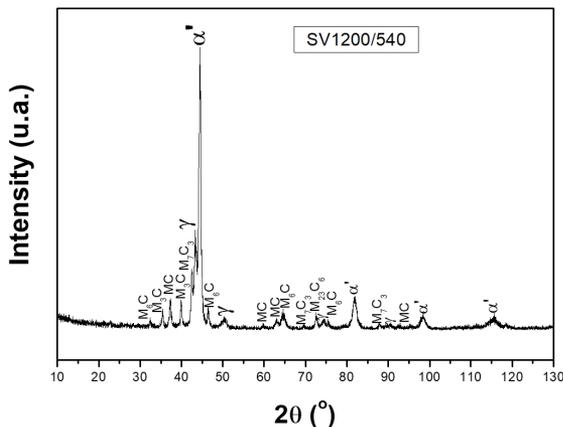
Figure 12. XRD of M3:2; 1200 °C/540 °C.
