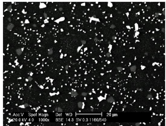
Figure 15. SEM of M3:2 + 0.3%C; 1160 °C/540 °C.
