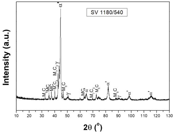
Figure 10. XRD of M3:2; 1180 °C/540 °C.
