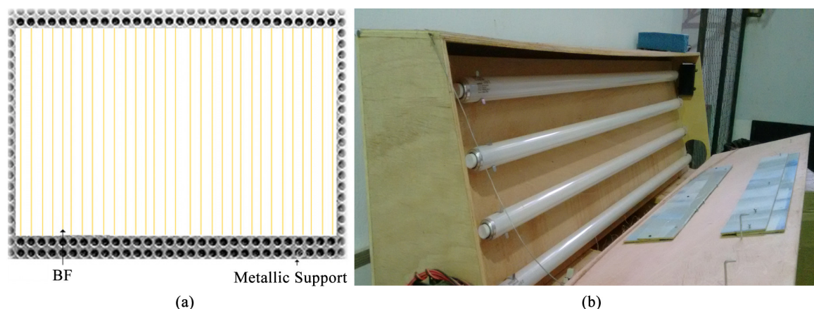
Figure 2. Apparatus used to apply UV radiation on BFs. (a) Representation of the metallic frame to keep the fibers aligned during exposure. (b) Photobleaching chamber build based on ASTM D5208-09 [13] . Bibliographic source: Author.
