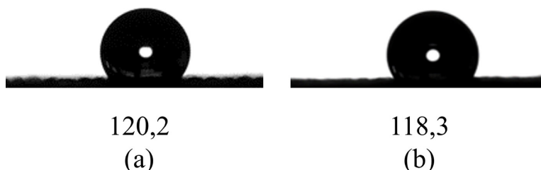
Figure 9. Contact angle of samples treated with (a) 2 and (b) 4 passages in the silica deposition process.
