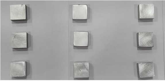
Figure 9. Before and After corrosion test samples of AT3, AT6 and AT9.
