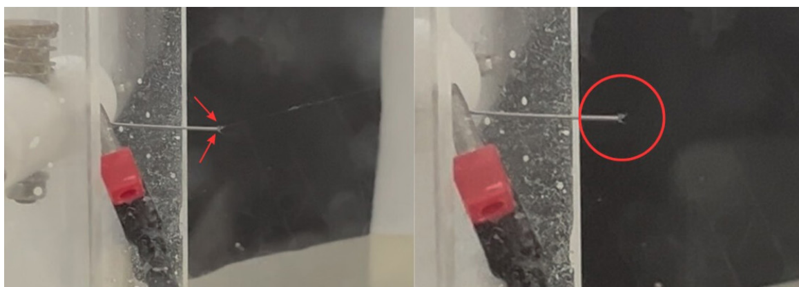
Figure 10. Taylor cone defects during the electrospinning process.
