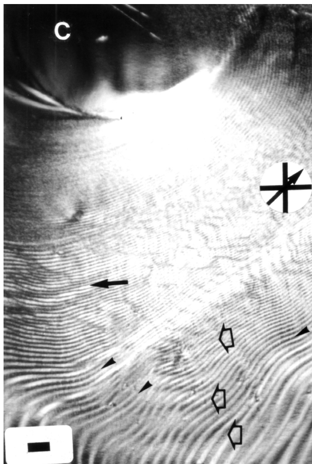
Figure 1. Birefringence image of the superstructure resulted from crystallization of two drops of PBLG solution in contact with each other as seen after Sénarmont's compensation. Compensated columns or cords appear black (arrow head), whereas non-compensated ones appear bright. The alternate compensation of the cords reveals their antiparallel molecular arrangement. The cords were positioned at 45 degrees with respect to the polarizer. The crossed lines indicate polarizer and analyzer azimuths, and the arrow indicates the respective statistical direction of the cord axis. Some degree of intertwining of cords due to changes in their direction is shown (arrow). These changes also reveal undulations (short empty arrow). C, center of one of the drops. Bar, 100 \mu\text{m} .
