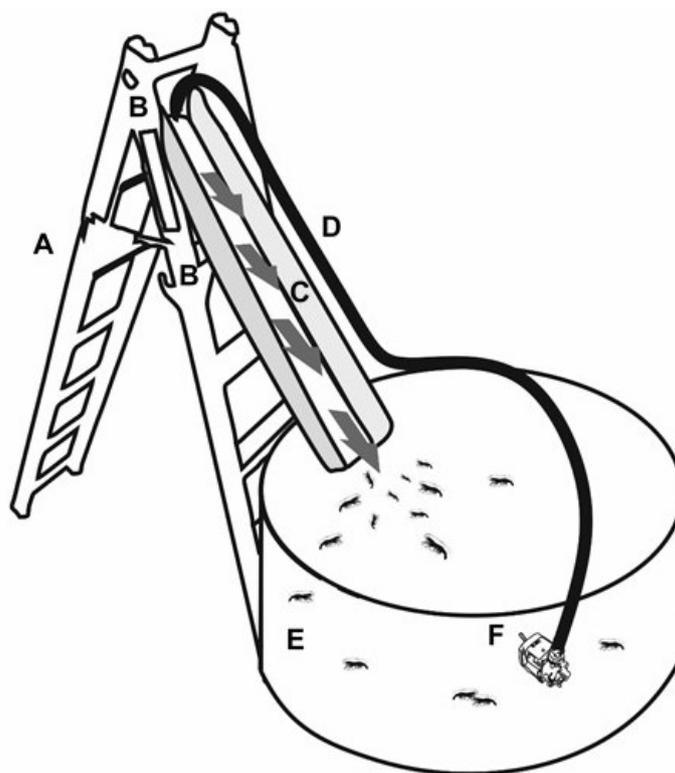
**Figure 1.** Experimental system used for migratory behavior bioassays of *Macrobrachium tenellum* juveniles. (A) support structure; (B) supports to adjust inclination; (C) galvanvanized metal channel with internal gutter of 10 cm; (D) water flow conducting hose; (E) circular tank, capacity 400 L with V cut; (F) submersible pump.
