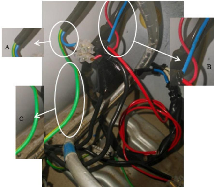
**Figure 3.** Image A: Power cable. Image B: neutral wire of the refrigerator's internal equipment in blue and 220 V phase wire in red. Image C: Ground wire.
