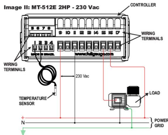
**Figure 4.** Rear interface of the temperature controller and the connections of the phase return to the refrigerator compressor. Adapted from the Full Gauge MT 512E 2HP temperature controller installation manual.
