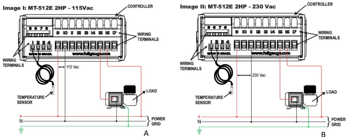
**Figure 2.** Rear interface of the temperature controller and the connections (circled in orange) for installation with voltage 110 V (A). Rear interface of the temperature controller and the connections (circled in orange) for installation in voltage 220 V (B). Adapted from the installation manual of the temperature controller Full Gauge MT 512E 2HP.
