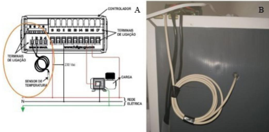
**Figure 6.** Installation of the temperature sensor: (A) connection of the temperature sensor to the temperature controller; (B) Extension of the sensor into the refrigerator. Adapted from the Full Gauge MT 512E 2HP temperature controller installation manual.
