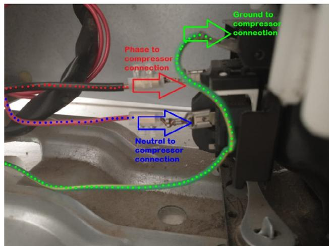
**Figure 8.** Phase wire (coming from the temperature controller) in black, neutral wire in red and ground wire from the power cable to the compressor in green.
