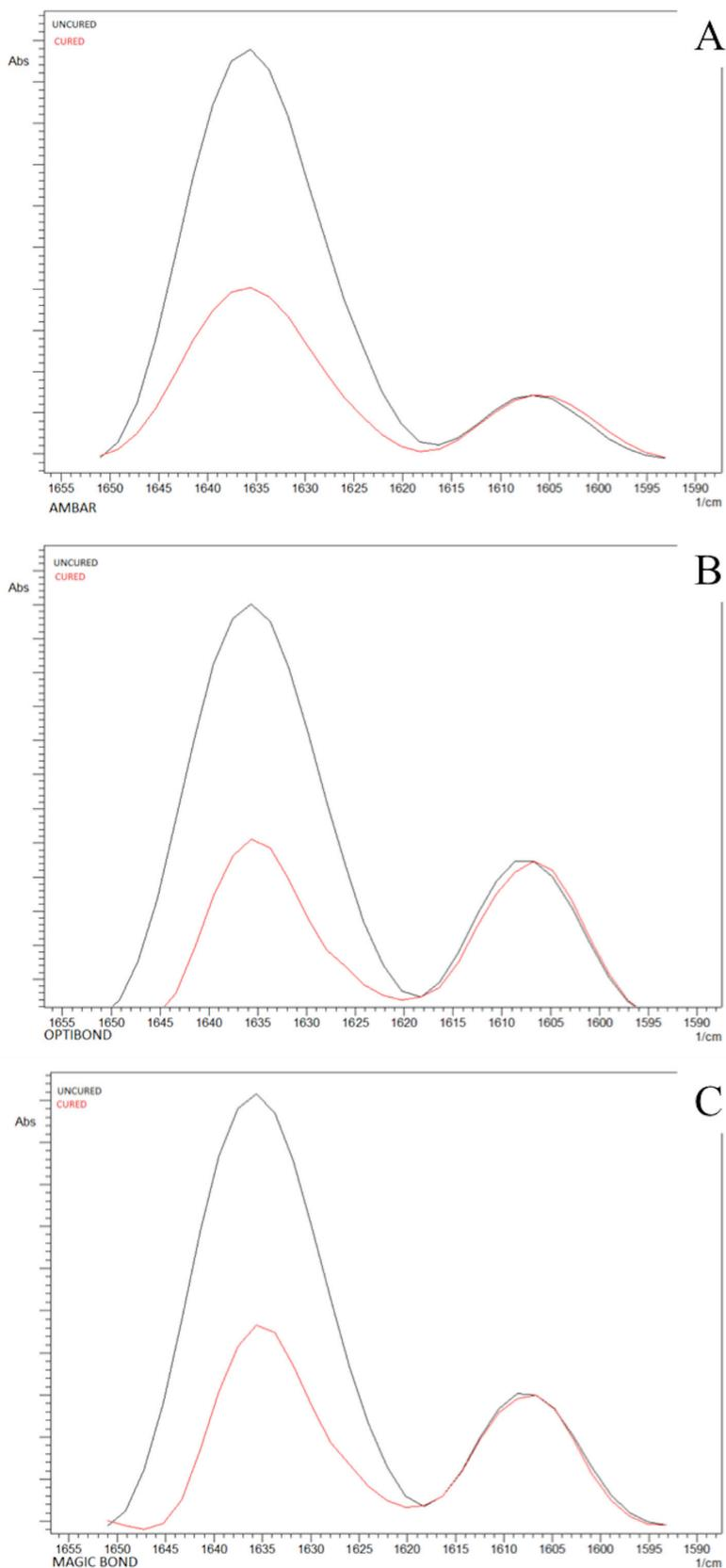
**Figure 1.** Fourier transform infrared spectra of adhesive systems. (A) Ambar; (B) Optibond; (C) Magic Bond,  $1638 \text{ cm}^{-1}$  = absorbance intensity for aliphatic carbon-carbon double bonds,  $1608 \text{ cm}^{-1}$  = internal reference for aromatic carbon-carbon double bonds.
