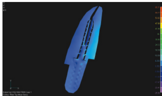
FIGURE 4 - Maximum tensile and compression stresses on the titanium Flexi Flange post.
