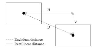
**Figure 1** – Representation of Euclidean (d = D) and rectilinear (d = H + V) distances.
