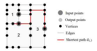
**Figure 4** – Grid with feasible flow paths for a problem with three facilities and contour distance  $d_{1,3}$  between the output of block 1 and the input of block 3 highlighted.
