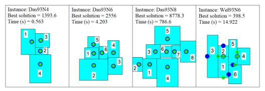
Figure 5 – Optimal layouts generated for fixed I/O points.
