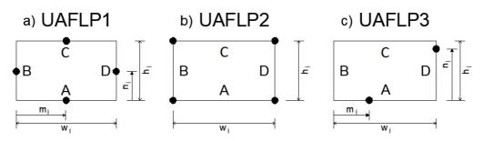
**Figure 2** – Departments with candidate locations for I/O points: a) four possibilities located on middle of the edges of the block; b) four options located on the corners of the block; and c) can assume infinite positions around on the boundaries of the block.
