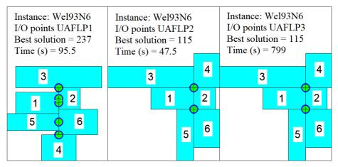
Figure 6 – Optimal layouts generated for variables I/O points.
