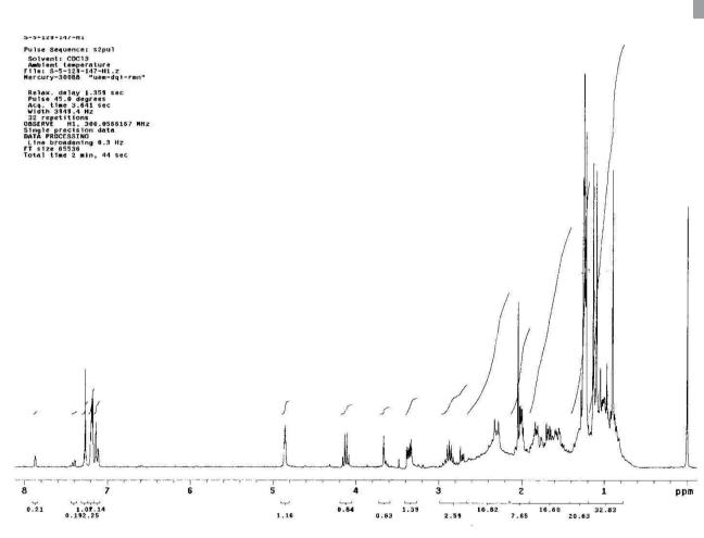
Figure 1S. <sup>1</sup>H NMR Spectrum of the compound 1 at 300 MHz in CDCl /TMS
