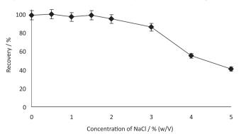
Figure 5. Effect of NaCl concentrations on the recoveries of Sudan Blue II ( $N=3, 0.5 \mu g mL^{-1}$  of Sudan blue II, pH: 4, volume of ethanol: 1.0 mL, volume of carbon tetrachloride: 125  $\mu$ L, centrifugation speed: 2500 rpm, time: 5 min)
