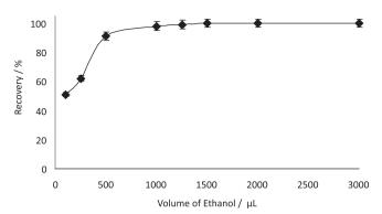
*Figure 3.* Effect of ethanol volume on the recoveries of Sudan blue II (N=3, 0.5 µg mL<sup>-1</sup> of Sudan blue II, pH: 4, centrifugation speed: 2500 rpm, time: 5 min)
