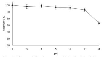
**Figure 2.** Influences of pH on the recoveries of Sudan Blue II (N= 3, 0.5 µg mL<sup>-1</sup> of Sudan blue II, centrifugation speed: 2500 rpm, time: 5 min)
