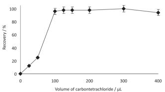
**Figure 4.** Effect of carbon tetrachloride volume on the recoveries of Sudan blue II (N=3, 0.5 µg mL<sup>-1</sup> of Sudan blue II, pH: 4, volume of ethanol: 1.0 mL, centrifugation speed: 2500 rpm, time: 5 min)
