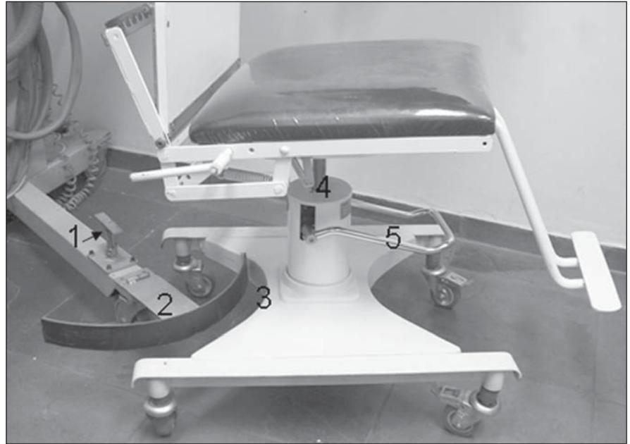
**Figure 3.** On 1, threaded insert for compensation of floor irregularities. Reciprocal fitting with convergent convex (2) and concave (3) surfaces. On 4, hydraulic axis. On 5, motion and locking lever of the hydraulic axis.
