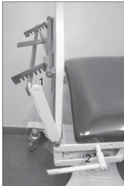
**Figure 4.** Double rack system, in which, with (1) angles between 90° and 60° can be achieved, and with (2) attachment under spring pressure, angles between 60° and 10° can be achieved.
