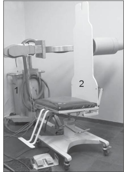
**Figure 1.** On 1, base of the C-arm. On 2, chair with hydraulic elevation, lowering and rotation mechanism to be fitted as an accessory of the radiological equipment.
