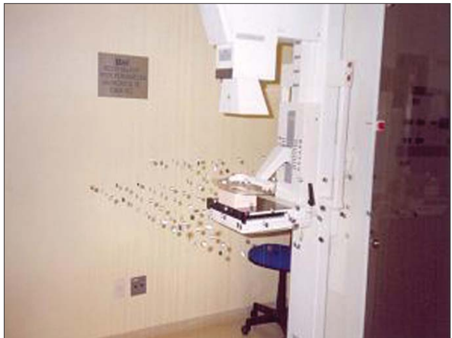
Figure 1. Photograph demonstrating dosimeters arranged around the mammograph with the breast phantom in place.
