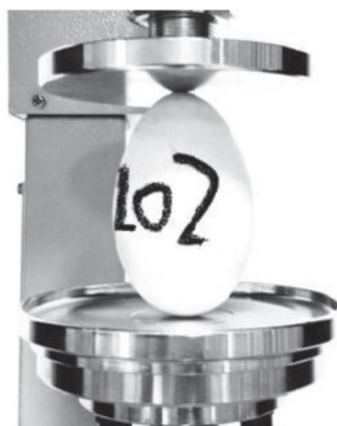
(b) Loading along the major axis.
