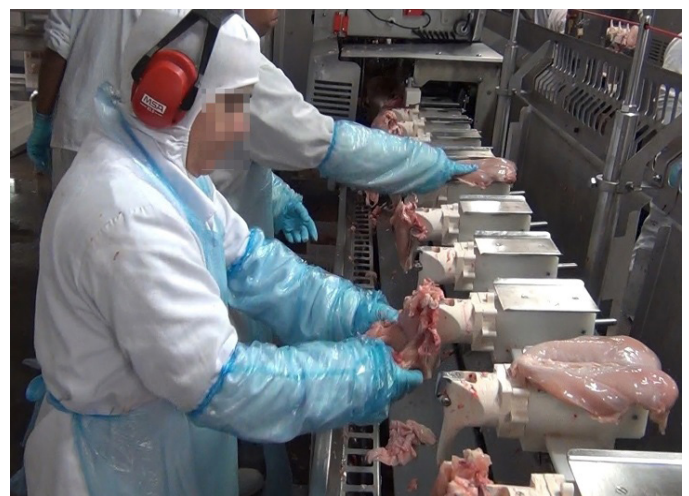
Figure 1 – Task of breast removal in deboning system sector.
